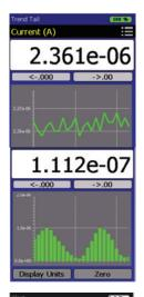
**Trend screen** has all the same features included in meter plus a large easy to read graph showing the readings over time. The graph can be displayed in bar or line graph format. Trend Tall
